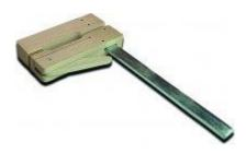
These clamps are constructed for use where a metal clamp is too heavy. The jaws are made of beech and the pressure pads are protected with cork to prevent marring of delicate surfaces. Clamp body of galvanized steel. The sliding lower jaw locks with an easy and quick to use cam lever.
